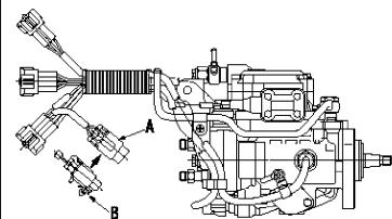
Q adjustment resistor clip assembly specifications
