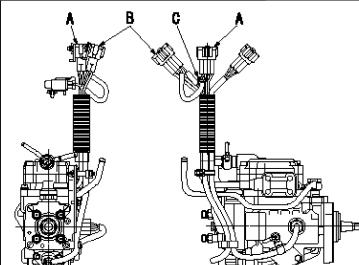
Q adjustment connector (harness) temporary fixing specifications
